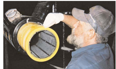
Thordon Composite EF bearings can be bonded or interference fit
