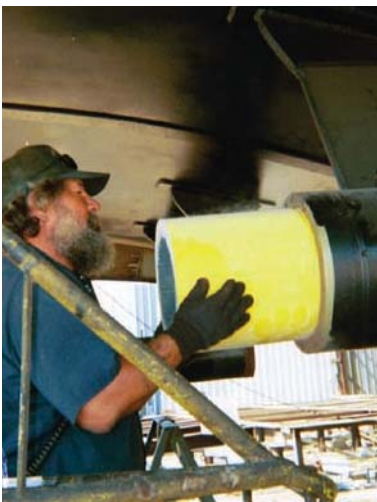
Easy Installation of Thordon Composite EF Bearing
